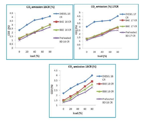
The carbon dioxide emission from the diesel engine with different blends is shown in graphs. The CO2 increased with increase in load conditions for diesel and for biodiesel blended fuels. The carbon dioxide emission from the diesel engine with different blends is shown in graph. The CO2 increased with increase in load conditions for diesel and for
